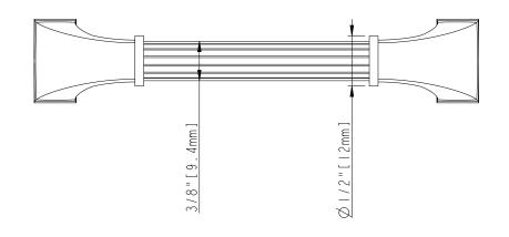
MATERIAL: Zamak 3 Z280 91.3 g/0.20 lbs PROPRIETARY AND CONFIDENTIAL THE INFORMATION CONTAINED IN THIS DRAWING IS THE SOLE PROPERTY OF HARDWARE RESOURCES INC. ANY REPRODUCTION IN PART OR AS A WHOLE WITHOUT THE DRAWN BY: Alexander.W Aug-06-20 APPROVED BY:
